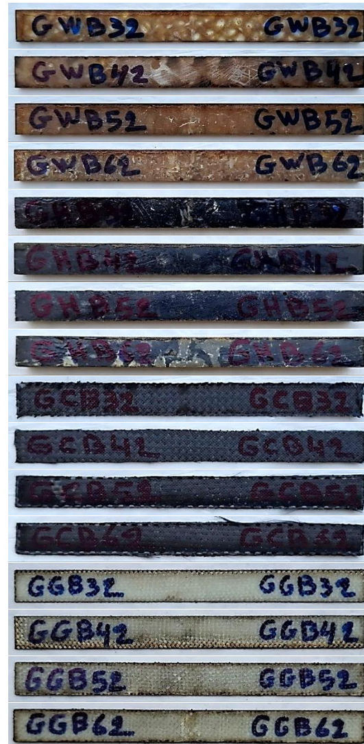
Figure 18. Flexural test specimens (sample 2)
