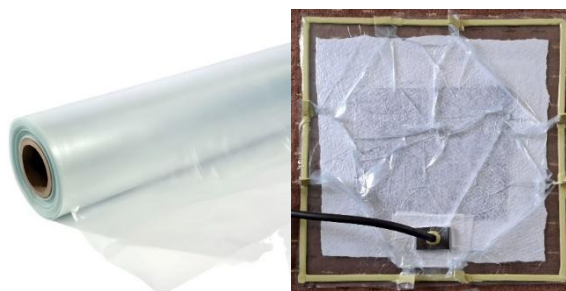
Figure 8. Multiple layers (plies) with bagging film
