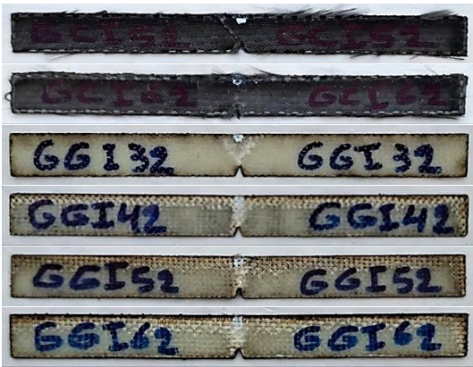
Figure 20. Impact test specimens (sample 2)
