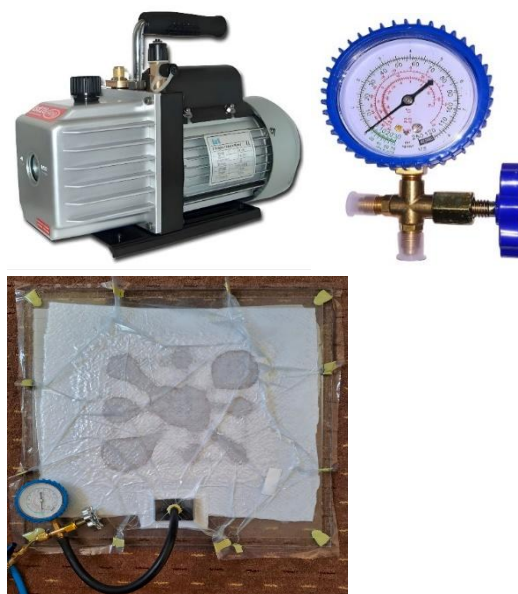
Figure 9. Multiple layers (plies) after vacuum Bagging
