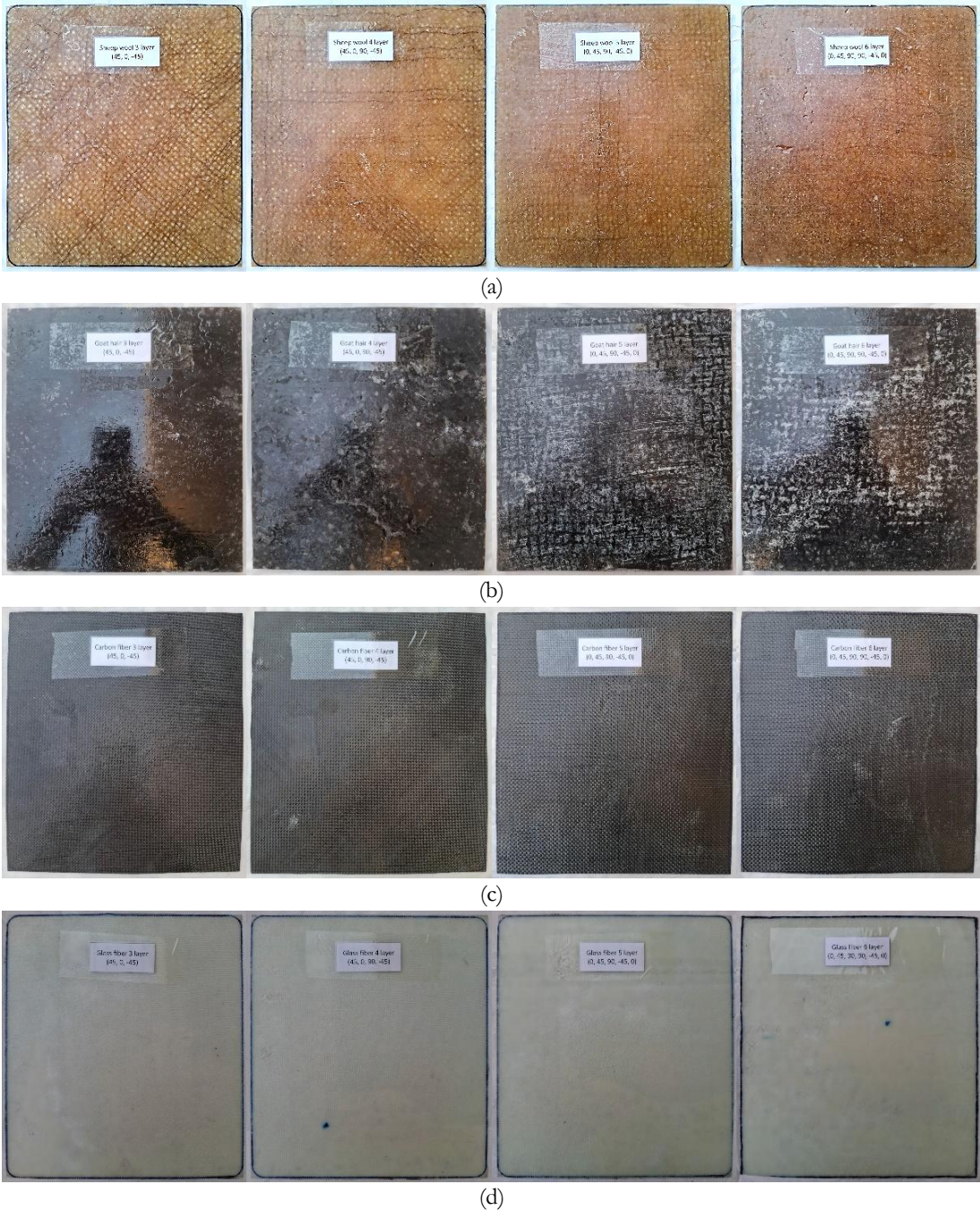
Figure 10. Multilayer (a) sheep wool, (b) goat hair, (c) carbon, (d) glass) fiber composite laminates
