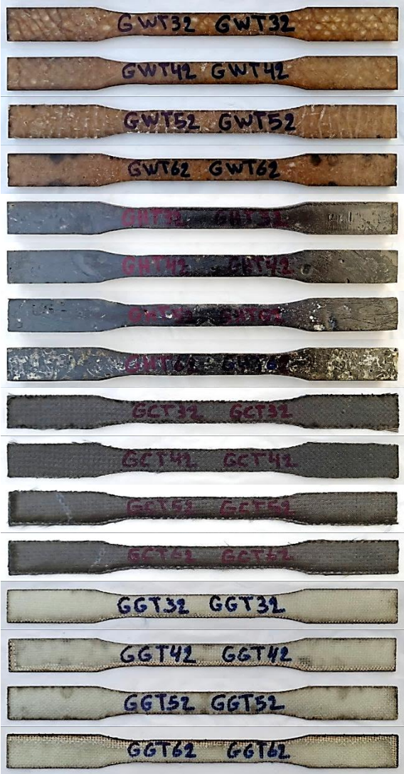
Figure 13. Tensile test specimens (sample 2)
