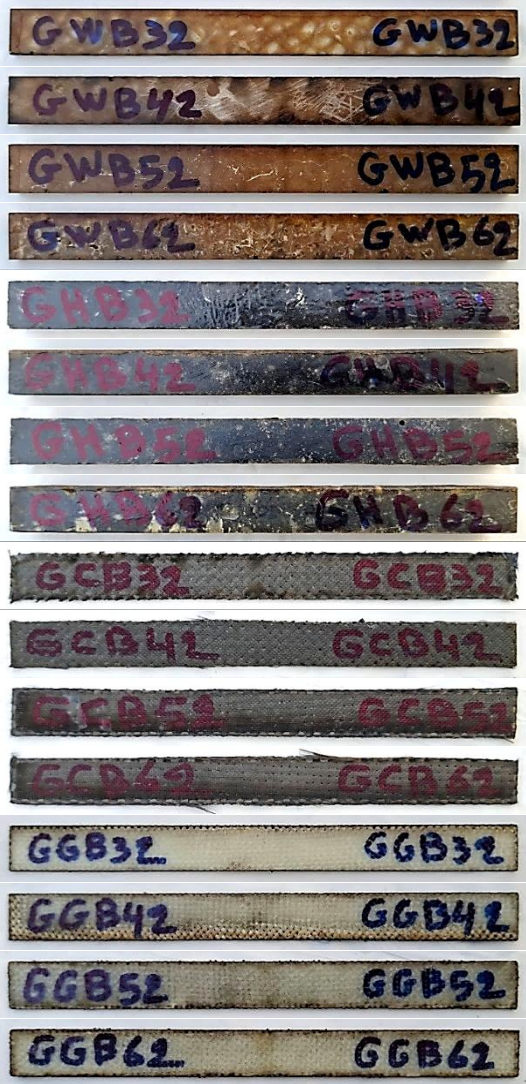
Figure 14. Flexural test specimens (sample 2)
