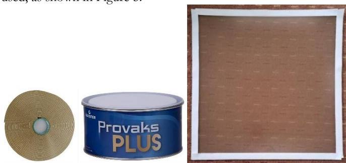
Figure 5. Glass mold preparation showing application of sealant tape and mold release wax
