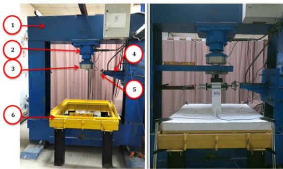
Figure 4. Test setup and components of testing, 1) Steel frame 2) Vertical actuator 3) Vertical load cell 4) Lateral actuator 5) Lateral load cell 6) Support of the specimens
