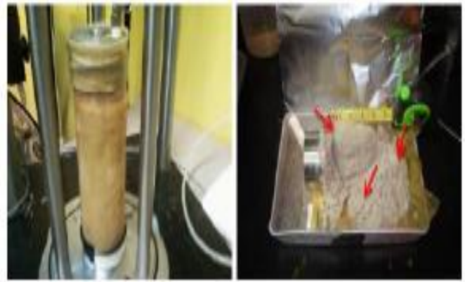
Figure 6. Triaxial sand column standing without support with a weighted stainless steel top-cap (left), a large strongly cemented center and several broken pieces found after CD testing (right) [13].
